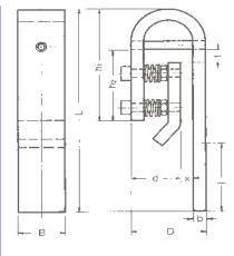
The **ERKO**® contact head FK is pushed onto the work or cathode rail from the top downwards. A flexible clamping plate presses the work rail against the contact surface of the head. The contact
