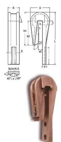
The **ERKO**® contact head is pushed onto the work or cathode rail from the top downwards. A clamping plate presses the contact surface of the head, via the wedge effect of the slideway guide, against the work rail, and thus establishes the non-positive contacting. The wedging can be easily released, either by the manual lever, which is pushed between
